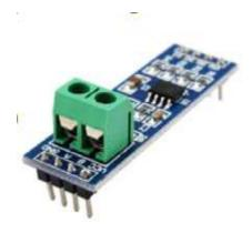
The modules makes it simple to use with microcontroller's UART to to create bidirectional RS485 networks.
